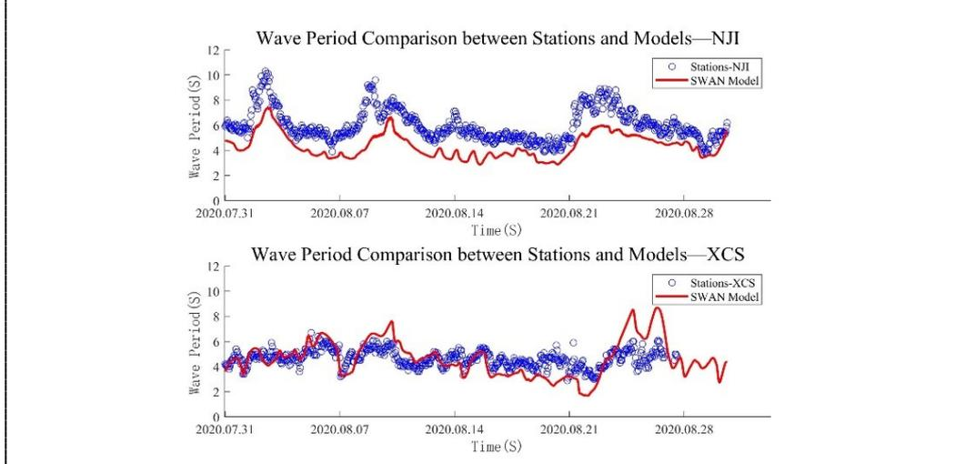
Figure 6. Wave period comparison between two data (NJI and XCS).
