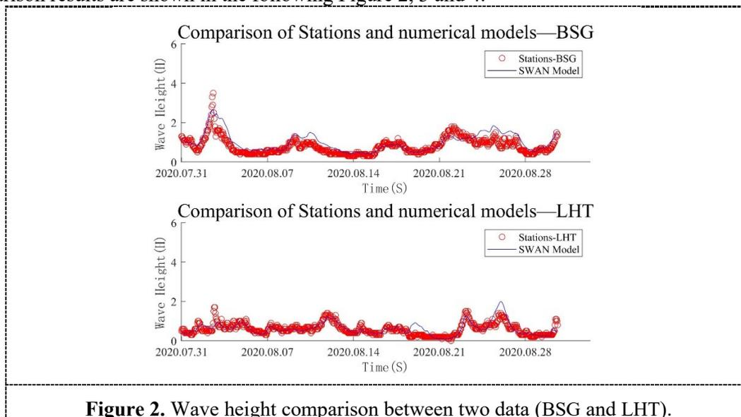
**Figure 2.** Wave height comparison between two data (BSG and LHT).
